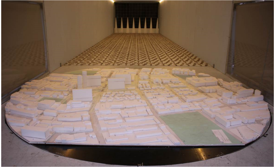
Figure 6d: Photograph of the Wind Tunnel Model – (View from the West)
